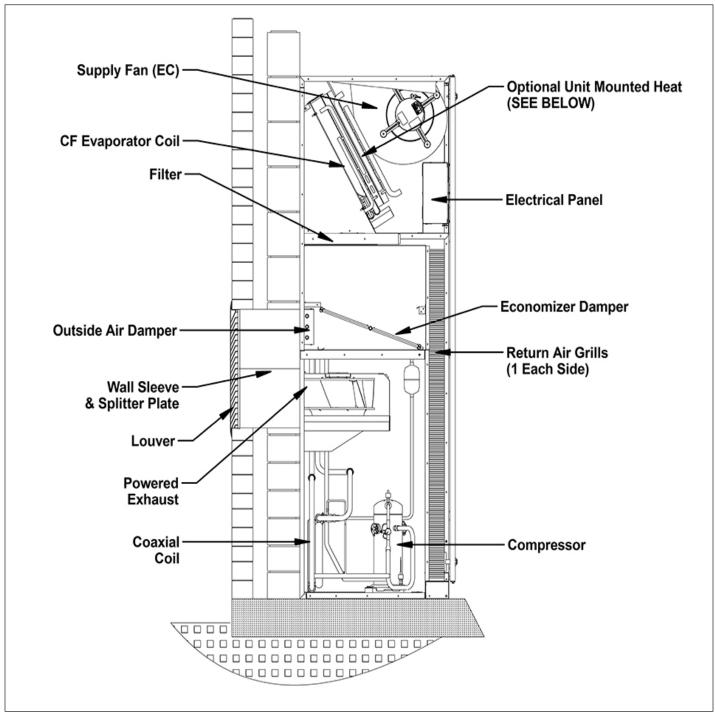
Unit shown with optional unit mounted heat, energy recovery wheel ventilation configuration with economizer damper, powered exhaust, single wall sleeve and louver. For project-specific general arrangement, contact your local sales representative for submittal data.
