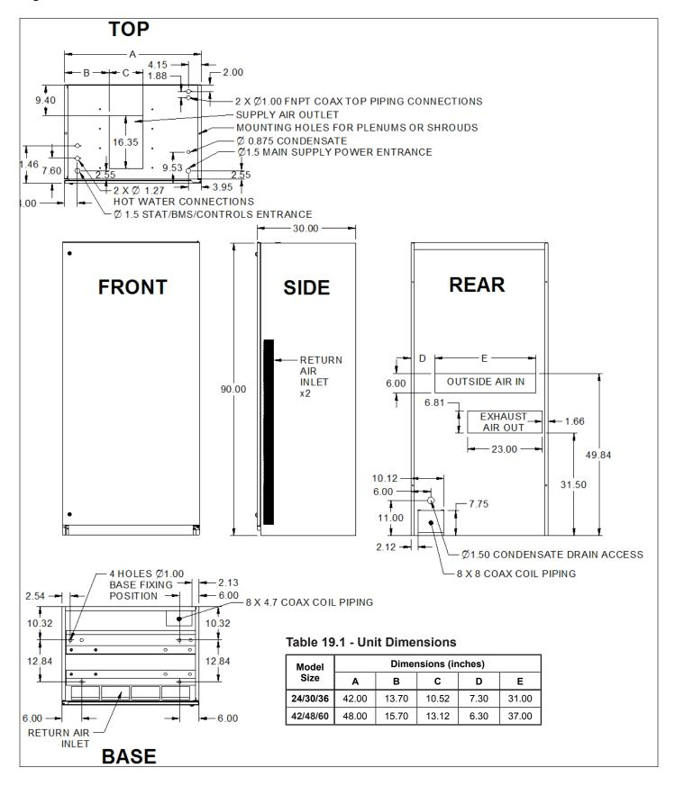
Figure 20.1 - Dimensional Data - Base Unit SMG & SMW with STUDY Package
