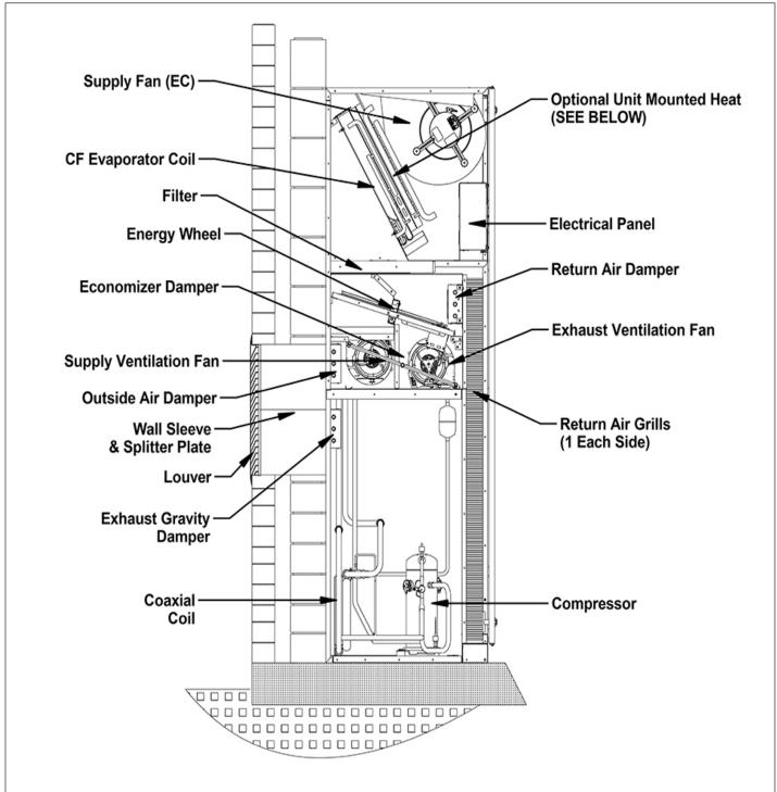
Unit shown with optional unit mounted heat, energy recovery wheel ventilation configuration with economizer damper, single wall sleeve and louver. For project-specific general arrangement, contact your local sales representative for submittal data.
