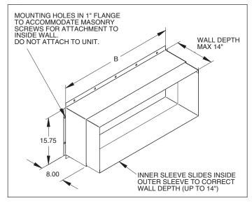
Figure 23.4 - Standard Wall Opening
