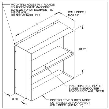
Figure 22.4 - Standard Single Wall Opening
